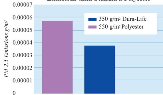
These flat sheet results are based on independent lab tests using ASTM D 6830-02 EPA PM 2.5 performance verification from the Environmental Technology Verification (ETV) Program comparing Durapex media from PGI vs. standard 550 g/m<sup>2</sup> polyester.
