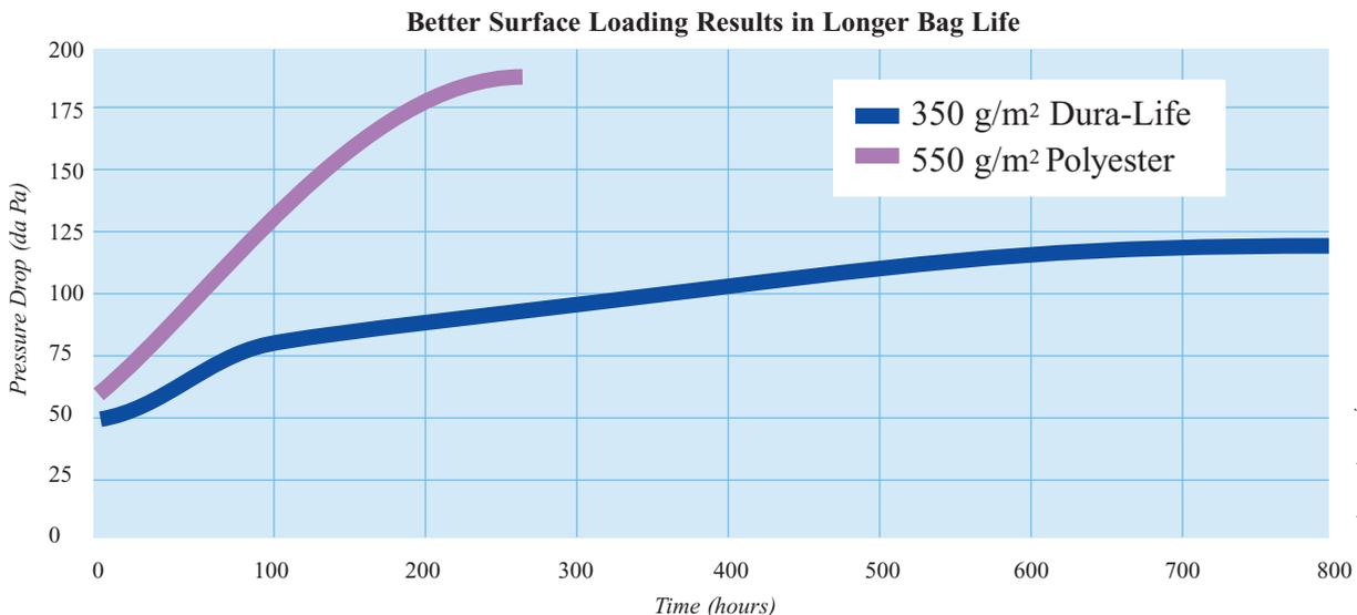
*These results were derived in accelerated lab tests, which correlate to field tests results, showing that Dura-Life will provide 2-3 times more life than standard 550 g/m<sup>2</sup> polyester bags in most applications.*
